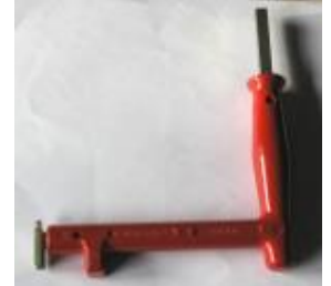
Slika 27: Pin extractor handle for taking off window sash
